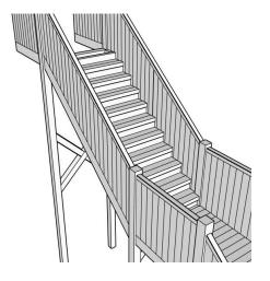
Fix the remaining risers and treads to the upper flight.
