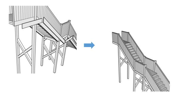
Finally, fix the two newel posts at the foot of the staircase as shown.
