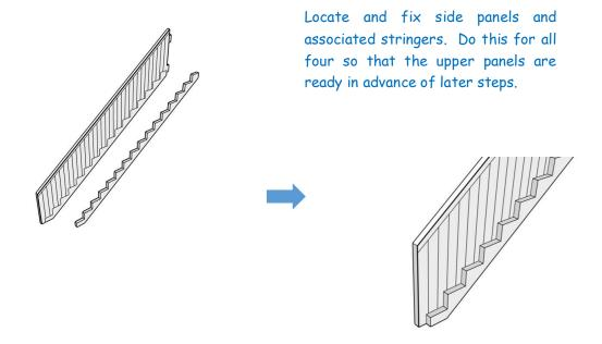
NOTE: Take care to make sure components are aligned correctly before they dry, misalignment may result in a poor fit or distortion to the staircase later.
