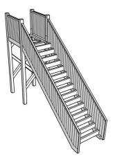
Fix risers to the remaining positions as shown.
