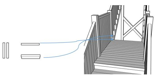
In a separate bag are a riser and tread shaped for the first step of the second flight. Fix them now in the location shown.
