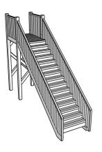
When the risers are set, fix all the treads as shown to complete the lower section.
