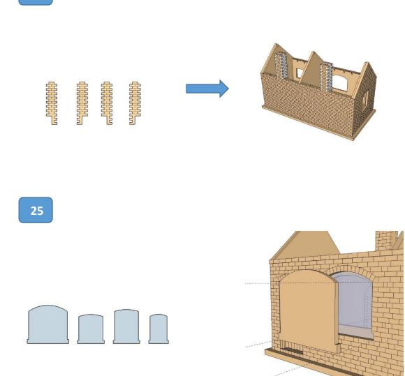
Identify glazing for each opening, use the blank window cut outs provided to press the glazing home evenly.
