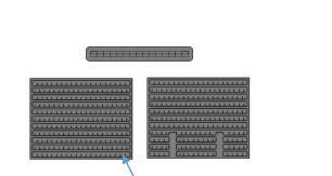
NOTE: Take the first row of tiles from the bottom of the sheet and start at the bottom of the roof.
