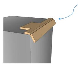
If the doors are to be represented in an open position carefully bend door hinges over a right angle prior to fixing them to the doors.
