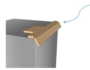
If the doors are to be represented in an open position carefully bend door hinges over a right angle prior to fixing them to the doors.
