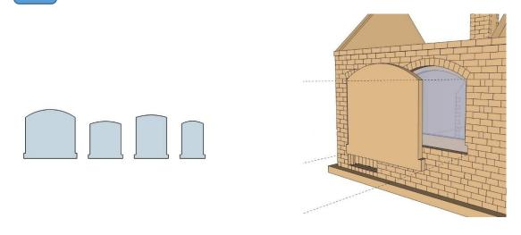
Identify glazing for each opening, use the blank window cut outs provided to press the glazing home evenly.
