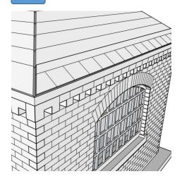
When fixing the roof tiles, use a small brush and apply PVA to the area you are going to fix the row of tiles. Observe that marks have been made on the tile underlay as a guide to where each row should go.
