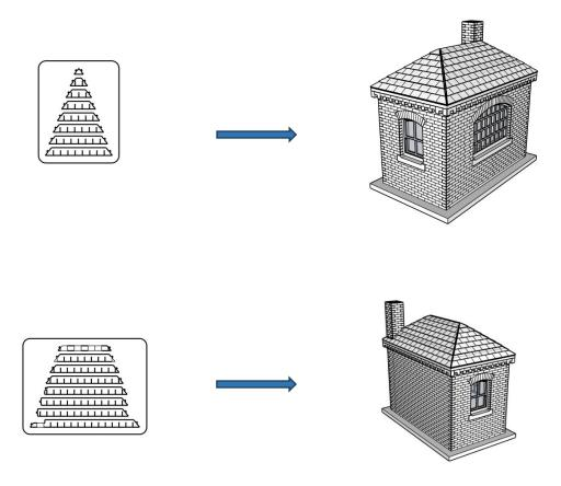
To finish the roof, locate the strips below. Release one part at a time. You will need tweezers for this, start by filling the relevant gap with a small amount of PVA, taking care not to spill over onto the tile surfaces. Place the strip in place.
