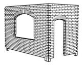
Begin by bringing together detailed brick wall parts applying adhesive at the brick joints. Be sure all the joins are square and the brick joints tight.
