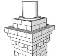
To complete the chimney, apply an appropriate amount of PVA on top of the previous assembly and site the pot. Any excess dried PVA will represent mortar.
