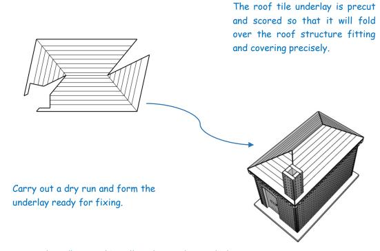
Apply adhesive liberally where the underlay makes contact with the roof structure. Pay particular attention over the eaves as you want the underlay to fit flush with the structure beneath. Work the underlay over the roof with your fingers as the underlay takes up the adhesive. You may need to keep pressure on for a short time.
