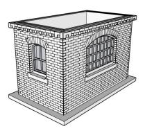
Locate and fix the eave detail by applying adhesive to top course of bricks.
